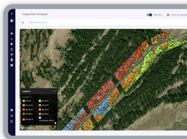
AiDASH analysis of vegetation around a transmission line. Image courtesy of AiDASH.
