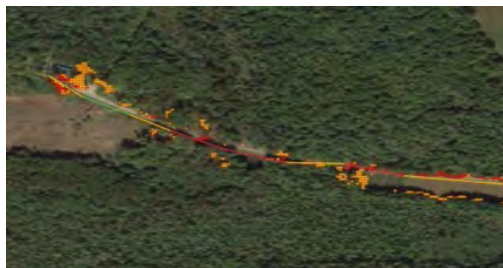
AI/ML evaluates and identifies unhealthy trees that may fall within right of way through woodland property.
